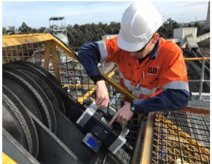
Residual MFL Wire Rope Inspection Set-Up.
